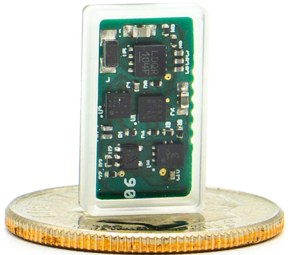
The most recent wireless version of the closed-loop vagus nerve stimulation device is about the size of a dime.
