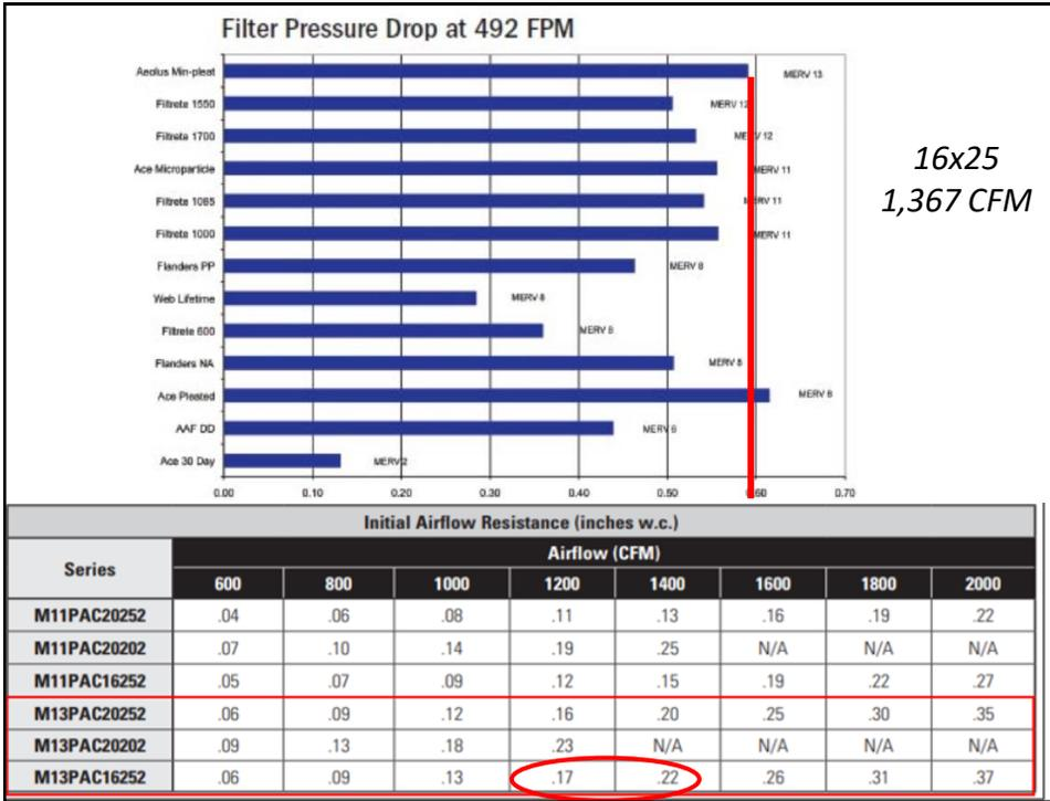
The York Affinity Hybrid air cleaner equates to a ~~Merv~~ Merv 16 (since it's a hybrid of media and electronic the rating system is slightly different), which means that it performs at the same level of a Merv 16. When you look at the airflow resistance in **Figure 7** (look at the blue line) and using 450 fpm as the guideline, we see that the Affinity filter has a pressure drop of only .13iwc.
