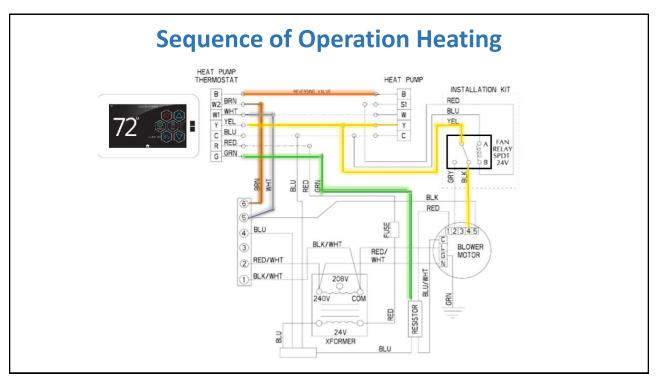
HMH7 with HMH7AK001Blower Relay Kit Installed
