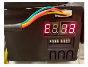
Fault Code 13 (Compressor Overheat Protection Device)
