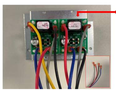
Wiring the RV relay
