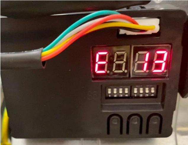
Fault Code 13 (Compressor Overheat Protection Device)
