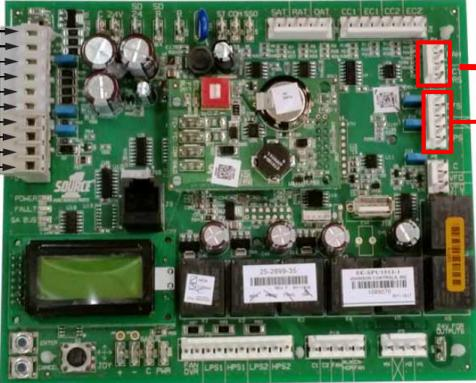
RAH= Return Air Humidity Sensor Input **0-10 VDC**
