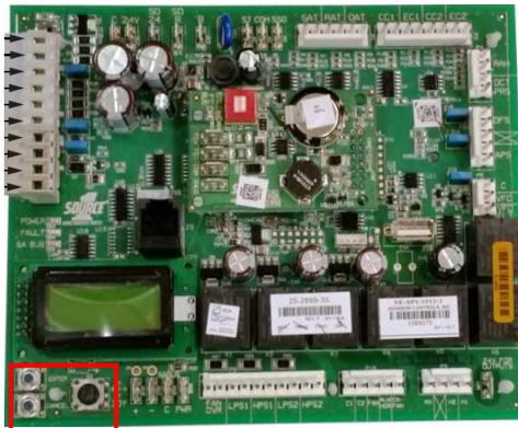
Up and down movement of Joystick will toggle between menus. Two selections will be on the screen. Cursor will be next to one of the menus. Side to side movement of Joystick will change selections within the parameter. Enter button will enter selected menus and save changes. Cancel button will move back one menu screen. May need to press multiple times to get back to home screen.
