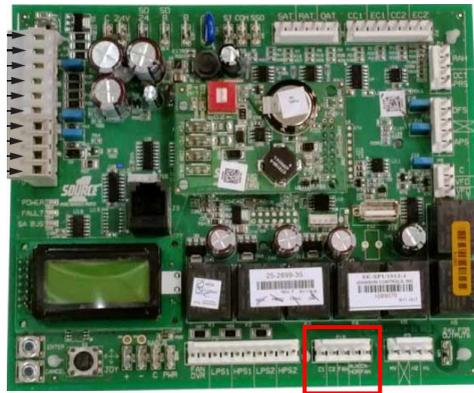
C1= Compressor #1 Contactor Output
