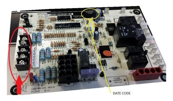
Note the red circle and arrow. This illustrates the missing 24VAC thermostat common connection. The location of control board date code is circled in yellow.
