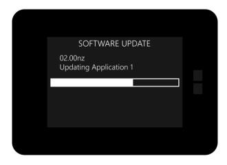
The Variable Capacity air conditioner and heat pump models must be controlled using the  $Hx^{TM}$  thermostat. The  $Hx^{TM}$  thermostat must have a front software version of 2.10nz or later to recognize and control these new models. The software update will be done **automatically** if the thermostat has a Wi-Fi internet connection.
