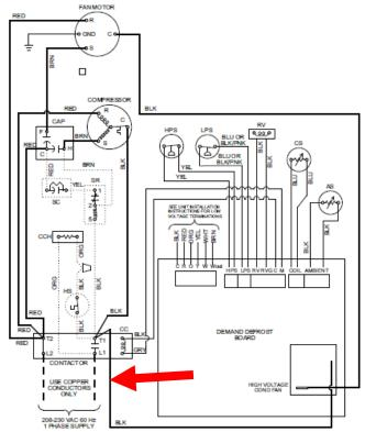
Implemented in August 2018, only the generation 2 YHE and RHP14L models were built with a true ECM motor, module, and wiring. Below is a wiring schematic showing where the ECM module's low voltage black wire is to be connected to the contactor 24 VAC coil.
