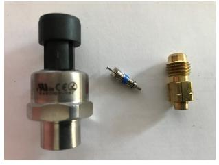
To install a flare type transducer in place of a sweat type transducer, the sweat type transducer must be removed and replaced with a brass <sup>1</sup>/<sub>4</sub> male flare connector like the one shown above. Since this is a brass to copper braze connection, a technician very proficient in brazing must make the repair.
