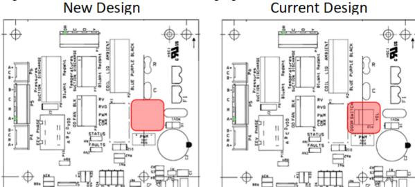
If a replacement control is installed in a field installed unit and the control does not contain the P12 connector, the unit door switch and YELLOW door switch wire harness should be removed and discarded.
