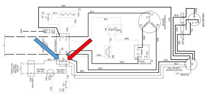
Some non-premium air-conditioning models have the motor controller control voltage wired in parallel with the incoming 24V A/C control voltage prior to connection with the contactor and the high and / or low-pressure switch. Using this wiring strategy, the outdoor fan motor should continue to operate even if a high-pressure event should occur, and the high pressure switch interrupted control voltage to the unit contactor. Test for 24V A/C at the locations shown below.
