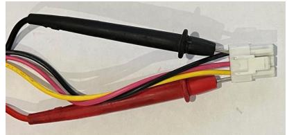
This method ensures a better meter connection to the windings. It also protects the integrity of the plug / socket connections. If testing from the other side of the plug, most likely the meter leads will damage the size of the connectors. An ohm reading across U - V, V-W, and U - W should be between 12 - 14 ohms. If outside of this range, condemn the motor. If an ohm reading difference between any two of the windings is greater than 0.3 ohms, condemn the motor.
