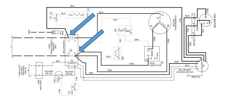
Next test is to check the control signal input to the motor controller. This must be done with an active cooling call. On a non-premium air conditioning unit, the motor controller control voltage input is typically wired in parallel with the outdoor unit compressor contactor low voltage. Test for 24V A/C at the locations shown below.
