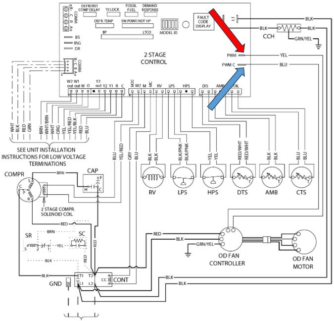
If a PWM capable digital multi-meter is not available, use the defrost control and its 7-segment display to visually
