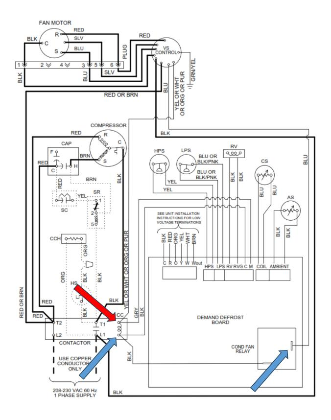
Most premium air conditioning and heat pump models utilize a variable speed outdoor ECM fan motor. The ECM motor controller is provided with a PWM (pulse width modulating) signal in lieu of 24V A/C. The PWM signal can be checked if a digital multimeter capable of reading such signal is available. Check the PWM signal at the locations shown below.
