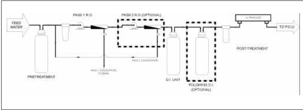
**Figure 1: Conventional Ultrapure Water Process**
