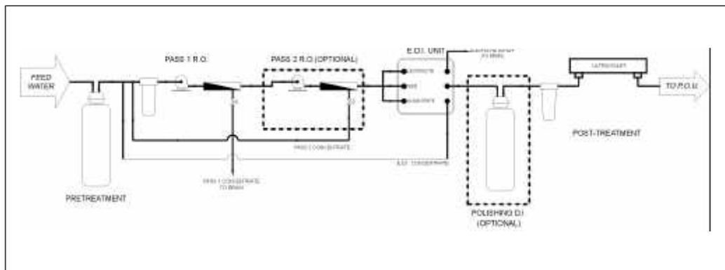
**Figure 3: RO/EDI Ultrapure Water Process**
