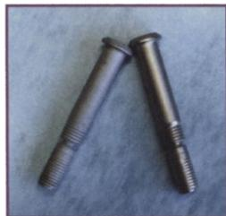
Figure 3: Titanium bolts before (left) and after (right) plating with electroless nickel.
