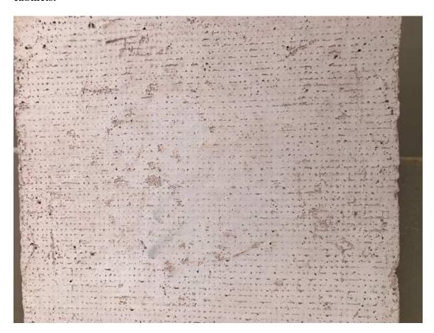
This picture shows a sample of a 1 sq.ft. piece of the composite mineral foam with an open web mesh embedded in the face. The mesh provides for a flat, glue-ready surface, ideally suited to the use of a latex adhesive or a moisture-cured urethane adhesive.
