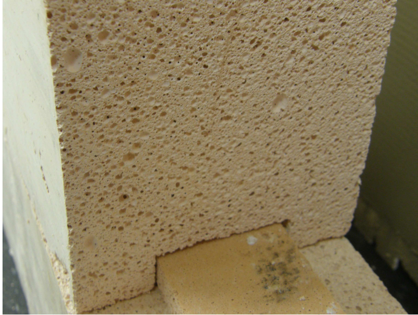
Note the mortis & tenon structure of the blocks for ease of installation.
