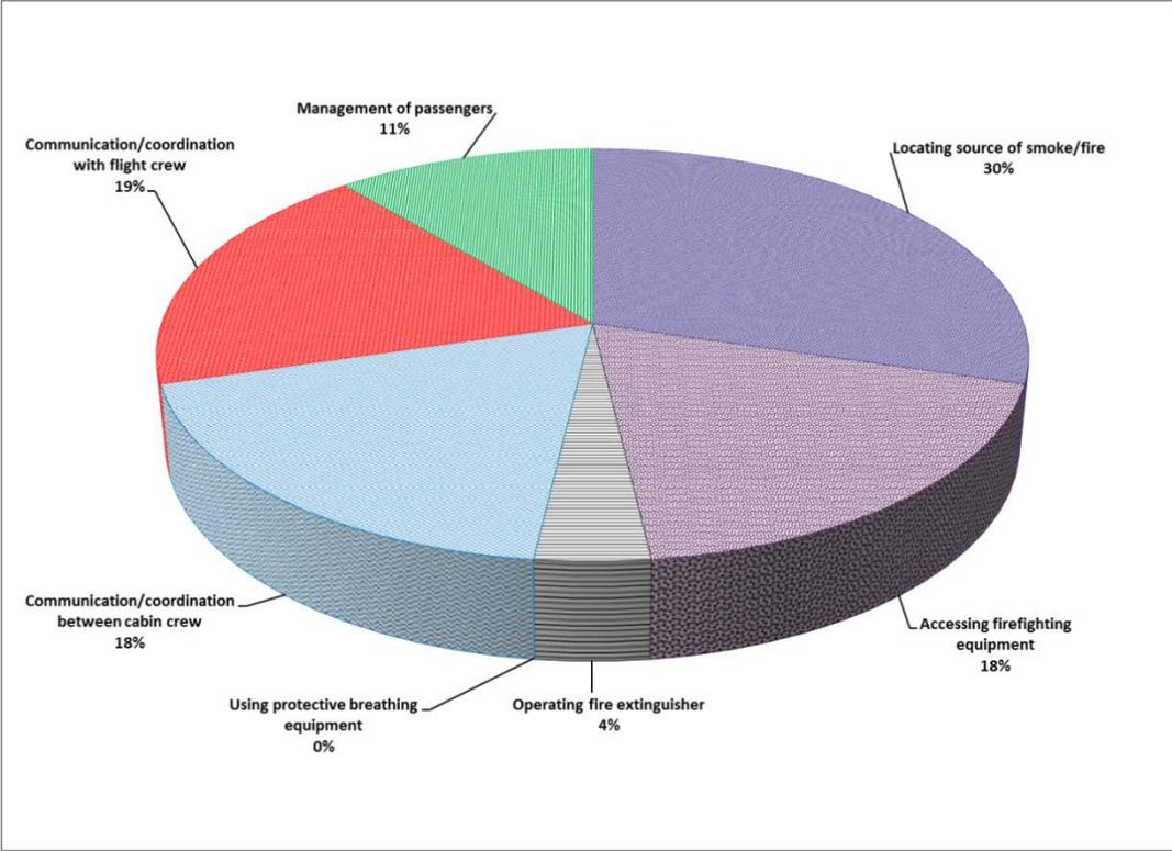
Figure 18. Problems encountered during in-flight firefighting
