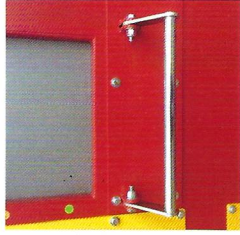
Real operating custom built heavy duty panic bar used with plunge cutting simulator.
