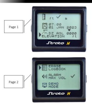
Use LB to navigate through the options. The left arrow (the selector) marks the current selection. Each LB press moves the selector to the next.
