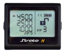
PF 3 is the Profille 3. Pressing RB sets the profiles: (RB) → PF1 (RB) → PF2 (RB) → (RB) PF3.
