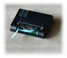
Bend the plastic stripe around the battery and close the battery compartment.
