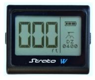
You can turn on/off backlight during climbing by pressing RB. When the feature is active, the LCD will automatically illuminate as soon as you leave the airplane and will be turned off after landing. The back light consumes a lot of power from the battery. So, avoid keeping it on during the aircraft climb.
