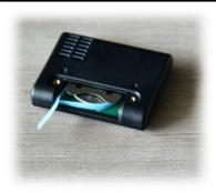
Bend the plastic stripe around the battery and close the battery compartment.
