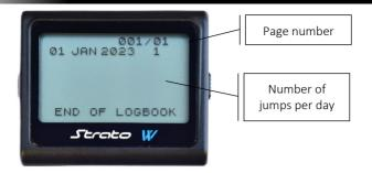
The altimeter can save up to 365(days) x 999(jumps/day) jumps. The log data of each day remains until the next(s) year(s). For instance, supposed the skydiver made five jumps on August 12, 2022. If the skydiver does not jump on August 12 of the subsequent years, the number of jumps save on August 12, 2022 will remain the same. On the other hand, if the skydiver did 2 jumps on August 12, 2023, the 5 five jumps saved on August 12, 2022 will be replaced by the 2 jumps done on August 12, 2023.
