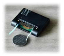
Install the new battery using the correct polarity.
