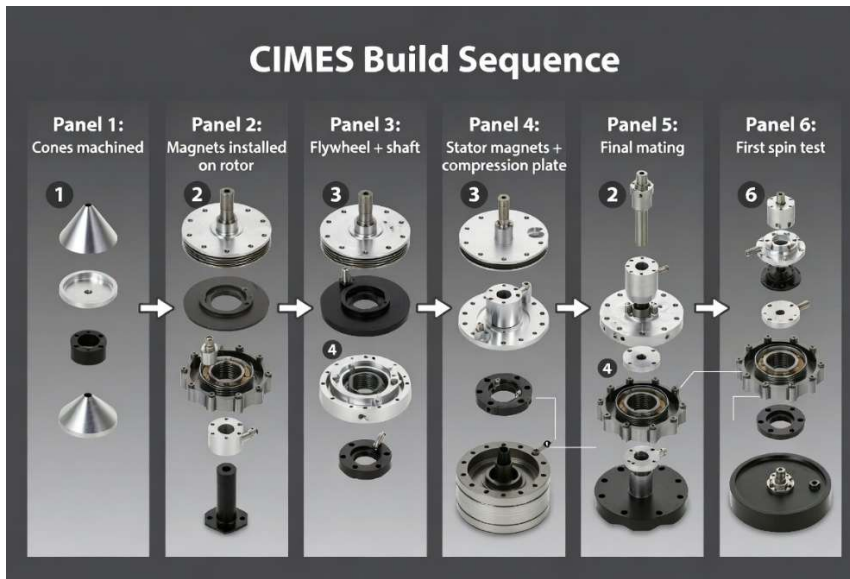
Figure 4 – Step-by-Step Assembly Sequence (6-Panel)
