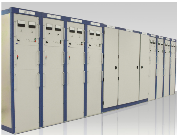
Eight 200 kW shipboard DTI PowerMod™ Power Supplies and 480 VAC power distribution providing 1.6 MW DC power for a radar transmitter.
