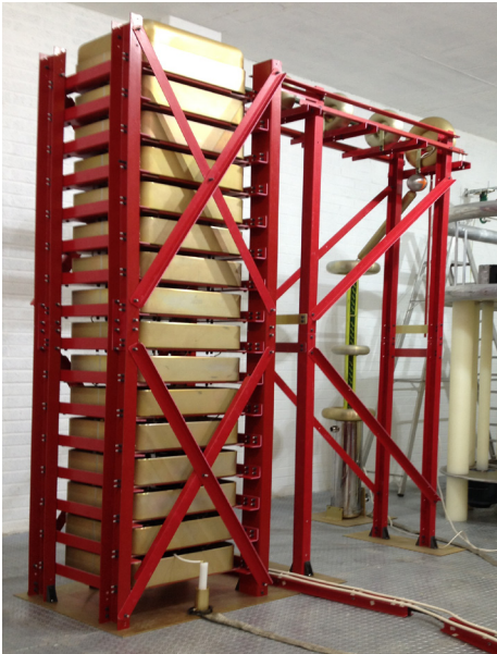
Custom DTI 400 kV, 400 mA DC Power Supply.
