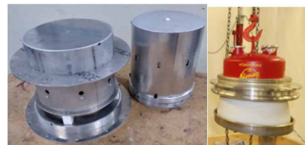
Figure 1: Surrogate tetrode made to the mechanical dimensions of the actual 4CM2500KG tetrode (left) and the added resistances to emulate the electron beam currents (right) photo of 2.5 MW high power 4CM2500KG tetrode.
