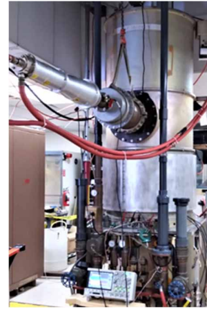
Figure 3: FPA assembly at DTI with short pulse water load attached to front coaxial output.
