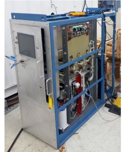
Fig. 2. Hybrid circuit breaker rated at 1 kV, 5 kA-continuous with mechanical contacts and modular solid state switch for 25 kA fault current. Module adiabatic thermal inertia allows network-coordinated interruption delays up to 50 ms; solid state switches interrupt in less than 1 ms. The breaker mechanically racks-out internal to the cabinet for galvanic isolation.
