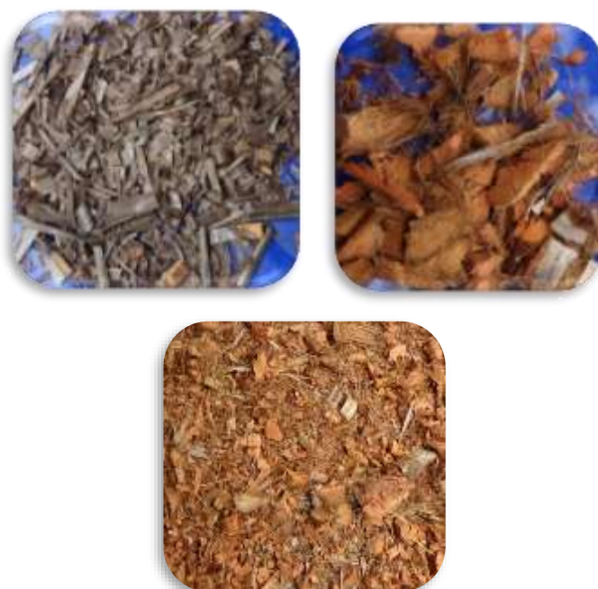
Fig. 2: Coconut sheaths/shells after shredding by Shredder
