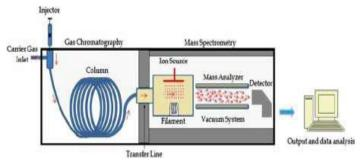
Principle of GCMS: A mixture will separate into individual substances when heated. The heated gases are carried through a column with an inert gas (such as helium). As the substances separated substances emerge from the column opening, they flow into the MS, it identifies compounds by the mass of the analyte molecule.
