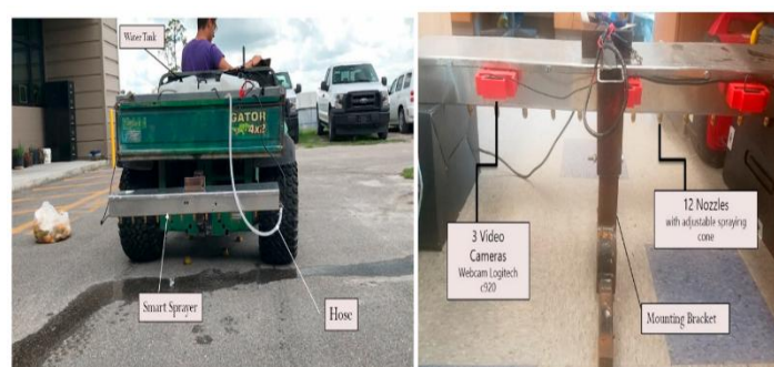
Fig 1: The Smart Sprayer mounted on an All-terrain vehicle (ATV) and main components of the Smart Sprayer
