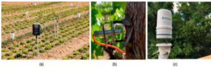
Fig.1: (a) soil sensors for irrigation scheduling, (b) plant sensor for detecting sap flow in plant stems, (c) ATMOS 41 for weather monitoring (source: Bwambale et al., 2023)
