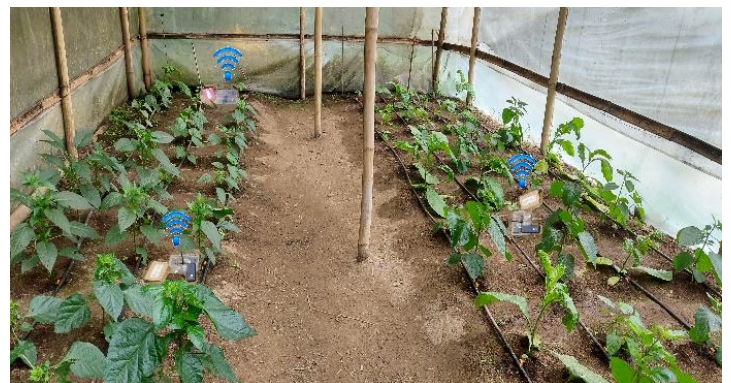
Fig. 2. Field view of IoT- based drip irrigation system inside the polyhouse
