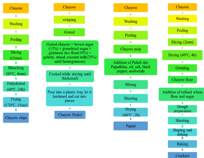
Fig 2: Process flow chart for Preparation of chayote chips, Dodol, Papad and Crackers
