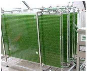
large illumination surface area. These are made up of transparent PVC materials for maximum utilization of sunlight
