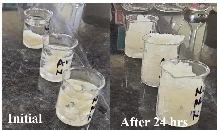
Fig 2: water swelling capacity of Nano Clay Polymer Composites after 24hrs
