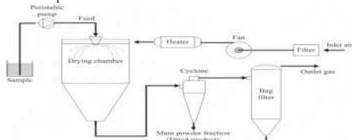
**A schematic diagram of the Spray Drier**
