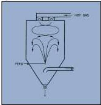
Dryers of this type combine both co-current and counter current flow. In a mixed flow dryer, the air enters at the top and the atomizer is located at the bottom. Like the counter-current design, a mixed flow dryer exposes the driest particles to the hottest air, so this design is not used with heat-sensitive products.
