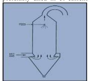
dryer offers more rapid evaporation and higher energy efficiency than a co-current design. Because the driest particles are in contact with hottest air, this design is not suitable for heat-sensitive products. Counter-current dryers normally use nozzles for atomization because the energy of the spray can be directed against the air movement. Soaps and detergents are commonly dried in counter-current dryers.
