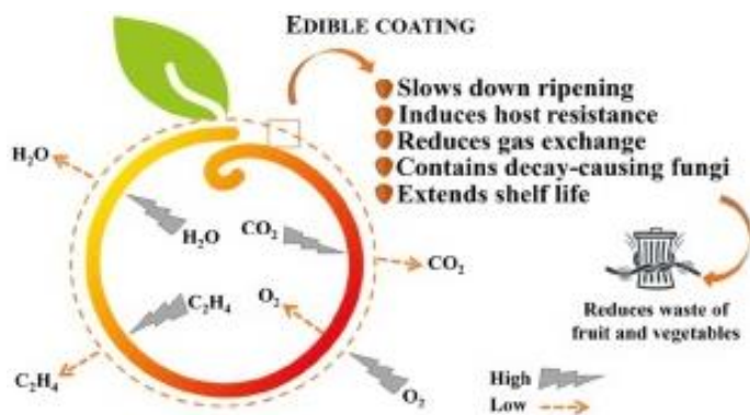
Fig 4. Mechanism and benefits of coating (Gianfranco and Marwa, 2022)
