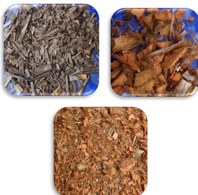
Fig. 2: Coconut sheaths/shells after shredding by Shredder
