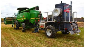
The Harrington Seed Destructor (HSD) was developed by an Australian crop producer, Ray Harrington, in 2005. The HSD is a trailer mounted cage mill with chaff transfer systems. Preliminary research using the HSD has shown that during commercial wheat harvest, 95 percent of annual ryegrass, wild radish, wild oat and bromegrass weed seed was destroyed (Walsh *et al.*, 2013).
