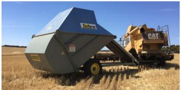
The simple chaff cart method consists of a chaff collection and transfer mechanism attached to a grain harvester that delivers the weed seed into a bulk collection bin. This method allows for the chaff and the weed seed to be collected and removed from the field. Another option is to dump the chaff material in the field and then burn the chaff piles. A drawback to this method is that the chaff cart attaches behind the already lengthy harvesting equipment, which makes
