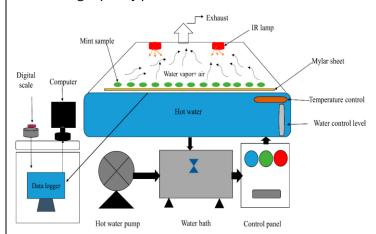
Fig. 1. Refractive window drying of foods Advantages of refractance window drying
