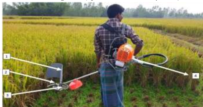
Fig. 1. Backpack-mounted brush cutter adapted for paddy harvesting. The unit features a crop guide (1) to organize stalks into windrows, a circular blade (2) for clean cutting, and safety guards (3) to minimize grain shattering. The backpack engine (4) provides stability on steep slopes. (Source: IndiaMART, 2024)
