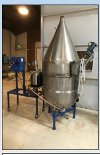
Pilot lignin cart to separate lignin from the CCR liquid fraction
