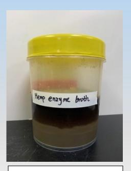
CCR pulp and sugars used to manufacture onsite cellulase enzymes
