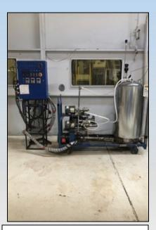
500-liter hydrolysis reactor to convert pulp into lactic acid
