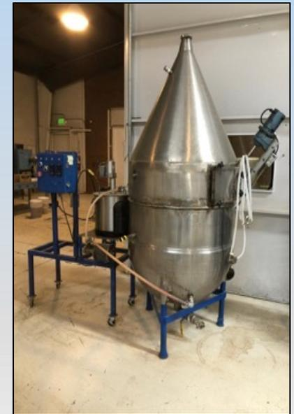
Pilot lignin cart to separate lignin from the CCR liquid fraction
