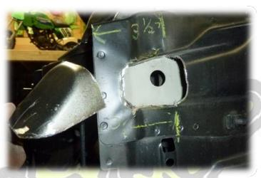
15. The area in front of the resulting hole must be reformed to properly fit headlights. See picture below, marked area (X) should be reformed with a hammer to make a concave area as viewed from front.
