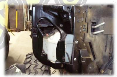
12. Drill Pilot holes with 11/32" drill bit if inserting Rivet Certs (Nuts and Bolts can also be used with washers in no rivet gun in available. Regular Aluminum rivets also create a clean look. Rivet Certs are Strongly Recommended for ease of installation and removal).
