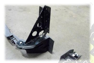
44. Bracket can now be mounted to radiator support using the two holes marked from the original template in earlier steps as pictured.
