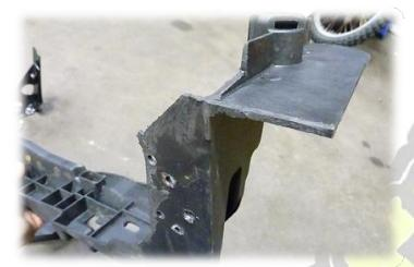
41. Once trimmed left and right lower head light / lower grill mount brackets can be installed as shown below
