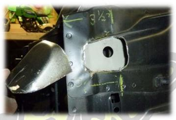
14. The area in front of the resulting hole must be reformed to properly fit headlights. See picture below, marked area (X) should be reformed with a hammer to make a concave area as viewed from front.
