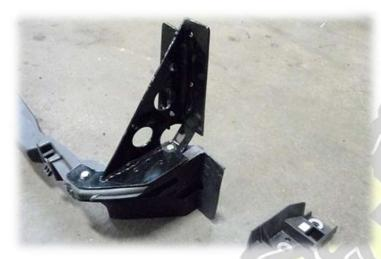
43. Bracket can now be mounted to radiator support using the two holes marked from the original template in earlier steps as pictured.
