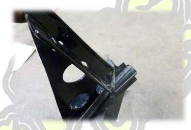
41. Place a bolt in the front bracket hole, through the factor plastic hole and hand tighten. More back holes can be drilled and install nuts and bolts per installers needs.
