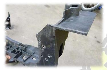
40. Once trimmed left and right lower head light / lower grill mount brackets can be installed as shown below
