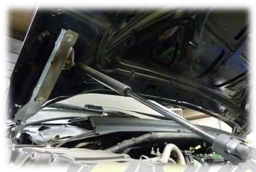
**NOTE:** Supplied washers may be used in place of factory shims. Do not expect factory shims to remain in same locations or be necessary. You may need more or less.
