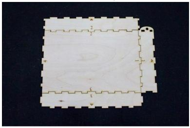
Glue and assemble Junctions 1 and 2 at the same time. This braces the parts against one another at a right angle
