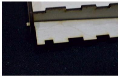
Glue and assemble Junction 4 inserting the hinge piece into the remaining axle hole so it moves freely
