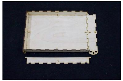
Insert the hinge piece labeled for Junction 5 into the axle hole of the partly assembled storage box (Do NOT place glue in axle holes)
