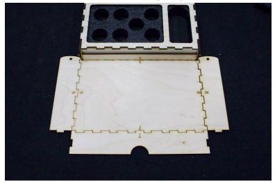
Glue and assemble Junctions 5, 6 and 8 Place a small drop of glue on both nubs of the hinge piece for Junction 5 (be careful to not saturate the axle hole)
