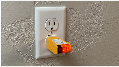
Test circuit for safe ground
