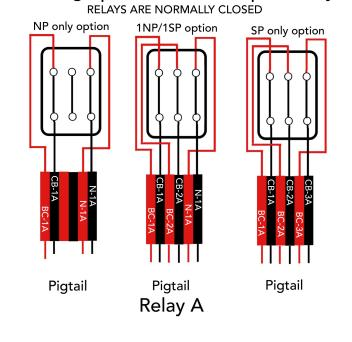
3 wiring options for each 3 pole relay
