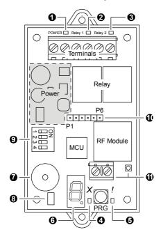
Remove top cover of the receiver to access DIP switches, beeper on/off jumper and antenna ports.
