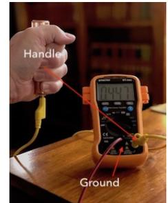
3. Plug the ground cord outlet connector into the electrical outlet (tested as safe and correctly wired as confirmed in step 1) in the room that the person is being evaluated in.
