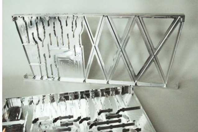
Satellite components are crafted using 6061-T6 Aluminum. Thin walled Wave Guides used for communications must be held within .001 over an 8" span
