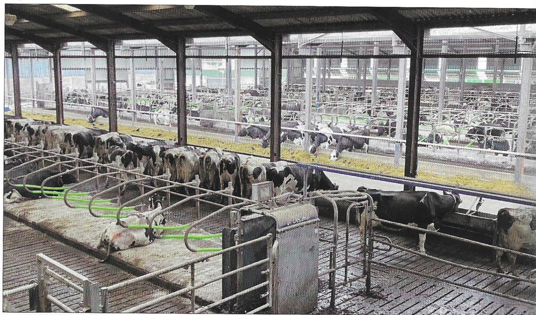
The nine robots are now milking up to 500 cows, producing an average of 2,600 litres/robot per day
