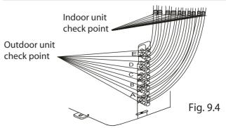
A, B,C,D are points for the one-four type. A, B,C,D, and E are points for the one-five type.
