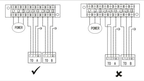
NOTE: Refer to the following figures if end-users wish to perform their own wiring. Run the main power cord through the lower line-outlet of the cord clamp.
