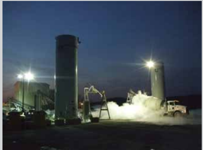
Night cooling with LN at a batch plant and generation of ground fog
